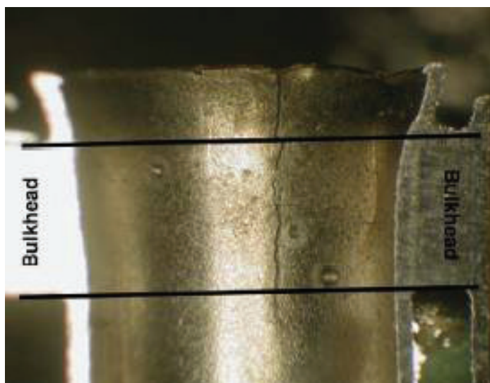
Close ups of a fatigue crack in a tube (above) and fin tube fatigue (left)
